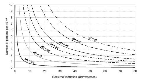
Fig. 4. Nomogram of number of persons per  $10 \text{ m}^2$  as a function of required ventilation rate per person, with the product of air change rate per hour (n) and room height (H) as a parameter (nH with unit m/h).
