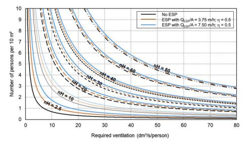
**Fig. 5.** Nomogram of number of persons per  $10 \text{ m}^2$  as a function of required ventilation rate per person, with the product of air change rate per hour (n) and room height (H) and the ESP characteristics as parameters (unit of nH is m/h).
