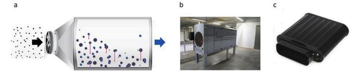
Fig. 3. (a) Concept of ESP with positive ionisation; (b) photo of moderate-size ESP ( $2.8 \times 0.72 \times 1.28 \text{ m}^3$ ) in an indoor environment. (Source: ENS Technology, reproduced with permission); (c) photo of small-size ESP ( $0.79 \times 0.40 \times 0.13 \text{ m}^3$ ) (Source: PlasmaMade, reproduced with permission).
